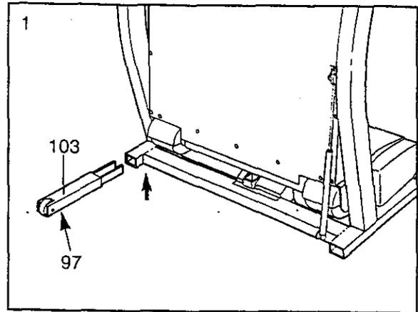
2. With the help of a second person, carefully lower the treadmill frame and then tip the Uprights (82) down as shown. **Make sure that the Extension Legs (103) remain in the Uprights.**
