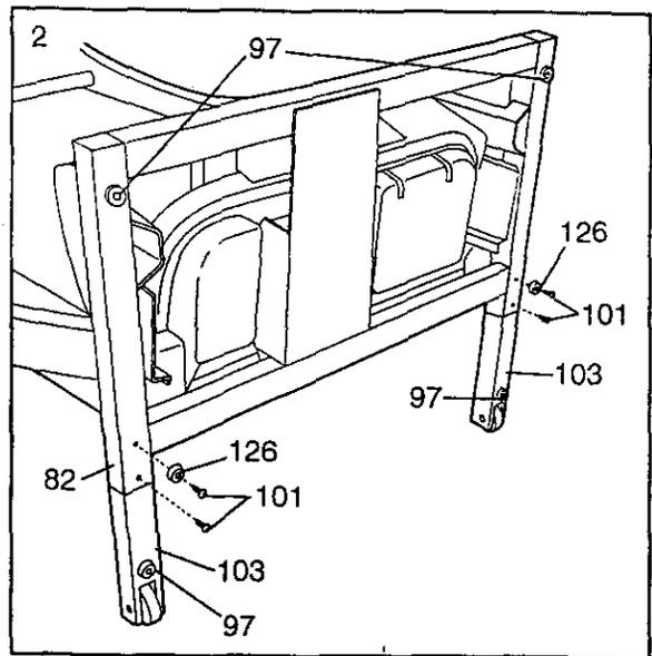
3. With the help of a second person, carefully tip the Uprights (82) back to the vertical position.
