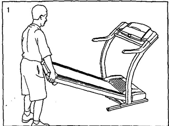
2. Move your right hand to the position shown and hold the treadmill firmly. Using your left hand, pull the latch knob to the left and hold it. Raise the treadmill until the latch pin is aligned with the hole in the catch. Insert the latch pin into the catch. Make sure that the latch pin is fully inserted into the catch.
