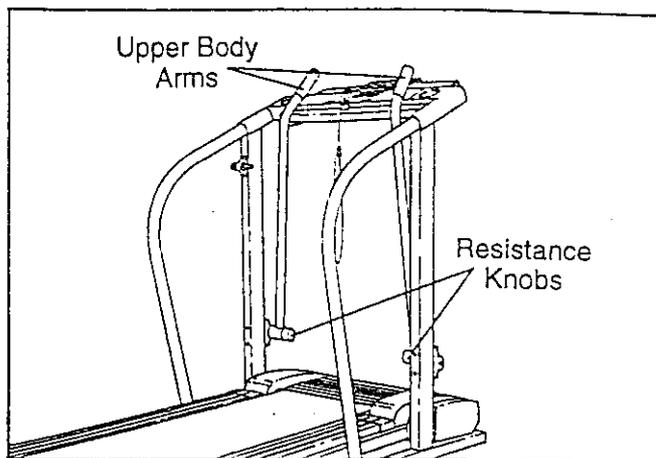
To vary the intensity of your upper body exercise, the resistance of the upper body arms can be adjusted. To increase the resistance, turn the resistance knobs clockwise; to decrease the resistance, turn the knobs counterclockwise.
