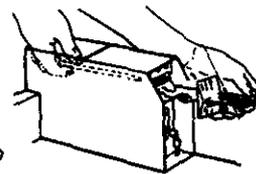
For dryers using coin slides, use adapter kit supplied with dryer.
