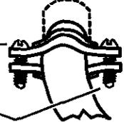
**8.** To exhaust dryer, see Exhaust requirements, Pages 3-4. Connect exhaust vent to dryer exhaust outlet and exhaust hood using 4" (10.2 cm) clamps. Use caulking to seal exterior wall opening around exhaust hood.
