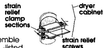
3. Assemble 3/4" U.L.-listed strain relief (U.L. marking on strain relief) into the hole below terminal block opening. Tighten strain relief screws just enough to hold the two clamp sections together. Install power supply cord/cable through the strain relief.
