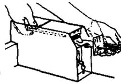
For dryers using coin slides, use adapter kit supplied with dryer. Replace the meter case service door. Put the coin vault with lock and key the meter case opening.
