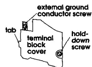
2. Remove hold-down screw and terminal block cover.
