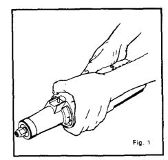
AWARNING: KEEP HANDS AND FINGERS AWAY FROM GRINDING AREA. ANY PART OF BODY COMING IN CONTACT WITH MOVING PARTS COULD CAUSE INJURY.
