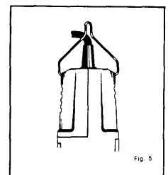
WIRE HANGER — (See Fig. 5). A wire hanger is provided for your convenience and ease of storage. To install, insert the ends of the hanger into the holes on each side of the grinder housing.
