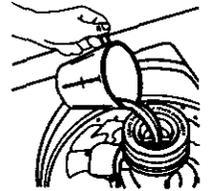
Dilute liquid fabric softener by filling the dispenser with warm water until liquid reaches the crossbar in the opening.
