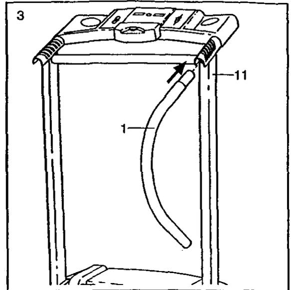
4. Align the hole in the Handrail (1) with the hole in the Upright (11). Tighten a Handrail Screw (53) two turns into the Upright and the Handrail (1). It may be helpful to lift up and down on the Handrail as you thread the Screw.
