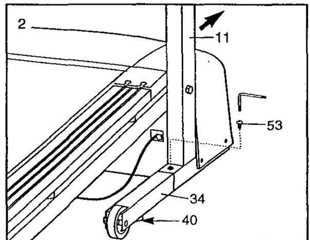
3. Insert the Handrail (1) into the tube at the upper end of the right Upright (11). Have a second person hold the Handrail as you complete step 4.
