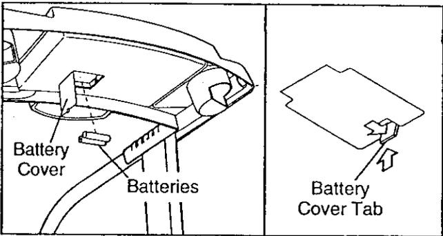
Close the battery cover, push up on the battery cover tab, and then push the tab forward as shown in the inset drawing. Be sure that the tab locks into place.
