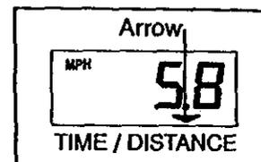
**CALS/FAT CALS/SPEED display**—This display shows the approximate numbers of calories and fat calories you have burned. (See FAT BURNING on page 14.) In addition, the display shows the speed of the walking belt, in miles per hour. Every seven seconds, the display will change from one number to the next, as shown by the arrows in the display.
