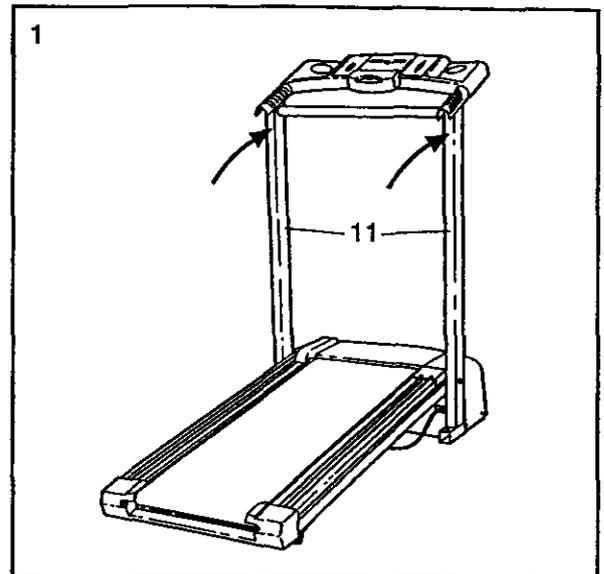
2. Insert one of the Extension Legs (34) into the treadmill as shown. Note: It may be helpful to tip the Uprights (11) in the direction shown by the arrow, as you insert the Extension Leg. Make sure that the Base Pad (40) is on the indicated side of the Extension Leg. Attach the Extension Leg with an Extension Leg Screw (53). Be sure to push on the head of the Extension Leg Screw while tightening it.
