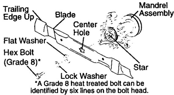
**IMPORTANT:** Blade bolt is Grade 8 heat treated.
