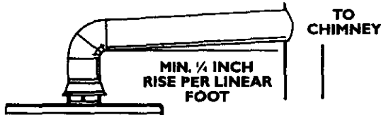
VENT PIPE INSTALLATION
