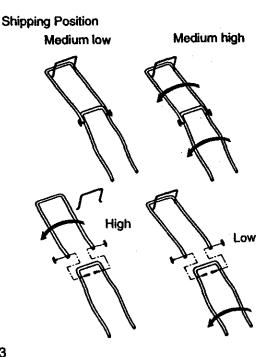
**CAUTION:** The operator presence control bar must pivot freely to permit blade/ brake engagement when control bar is released. Do not overtighten the fasteners holding the controls to the upper handle.
