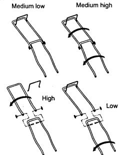
**ACAUTION:** The operator presence control bar must pivot freely to permit blade/ brake engagement when control bar is released. Do not overtighten the fasteners holding the controls to the upper handle.
