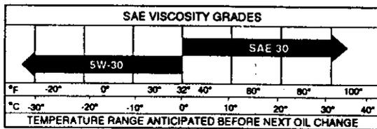
**NOTE:** Although multi-viscosity oils (5W-30, 10W-30, etc.) improve starting in cold weather, these multi-viscosity oils will result in increased oil consumption when used above 32°F (0°C). Check your engine oil level more frequently to avoid possible engine damage from running low on oil.
