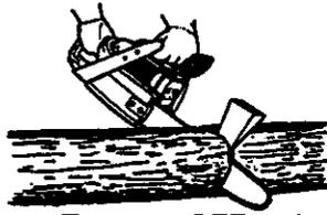
Turn saw OFF and use a plastic or wooden wedge to force cut open.
