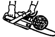
**Undercutting** involves cutting on the underside of the log with top of saw against the log. When undercutting use light upward pressure. Hold saw firmly and maintain control. The saw will tend to push back toward you.
