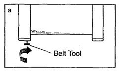
b. If the walking belt has shifted to the right, first remove the safety key and UNPLUG THE POWER CORD. Using the belt tool, turn the rear roller adjustment bolt counterclockwise 1/4 of a turn. Plug in the power cord, insert the safety key and run the tread-mill for a few minutes. Repeat until the walking belt is centered.
