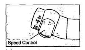
Carefully step onto the walking belt and begin exercising. Change the speed of the walking belt as desired by turning the speed control. To stop the walking belt, turn the control to "RESET."
