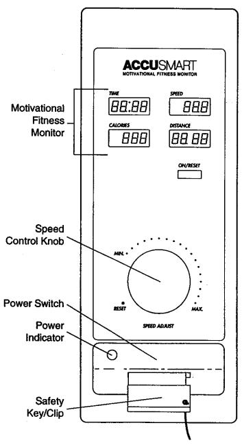
TIME—This display shows the elapsed time. Note: When the walking belt is stopped, the TIME display will go into a pause mode after a few seconds.
