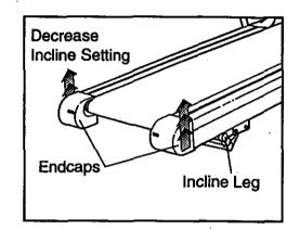
**A** CAUTION: Push slightly on the back of the treadmill to make sure that the incline leg is locked into one of the three incline settings before exercising on the treadmill.
