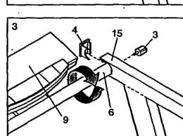
Slide the left end of the Console Crossbar (6) into the Left Upright (2). Tighten a Console Knob (3) into the Console Crossbar.
