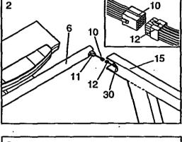
5. Plug the lower end of the Upright Wire Harness (12) into the 20" Wire Harness (45). The small latch on the Upright Wire Harness should snap onto the 20" Wire Harness (see the upper inset drawing). If the Wire Harnesses do not fit together easily, turn them; do not force the Wire Harnesses together.
