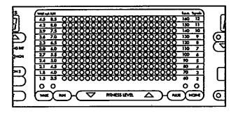
If you selected the WALK or RUN mode, red indicators will show the speed setting of each segment. If you selected the INCLINE mode, green indicators will show the incline setting of each segment. If you selected the WALK and INCLINE modes or the RUN and INCLINE modes, both red and green indicators will be lit.
