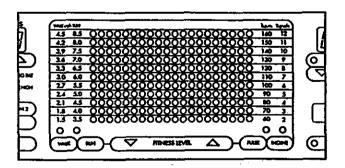
The settings of the first segment will be shown in the far left column, and the settings of the twentieth segment will be shown in the far right column. Red indicators will show the speed setting of each segment, and green indicators will show the incline setting of each segment.
