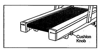
For a firmer cushion level, turn the knob clockwise; for a softer cushion level, turn the knob counterclockwise. Note: The faster you run on the treadmill, the firmer the cushion level should be. If the cushion level is too soft, the treadmill will bounce excessively.
