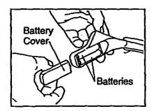
battery compartment showing which direction the batteries must be turned. Insert two batteries into the battery compartment. Close the battery cover.
