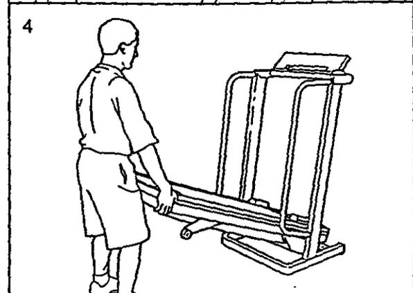
5. Move your right hand to the position shown at the right, and hold the treadmill firmly. Using your left hand, lift the Storage Latch (110). Raise the treadmill until the locking pin snaps into the Storage Latch. Make sure that the locking pin is inside the Storage Latch, and that the Storage Latch is fully closed.
