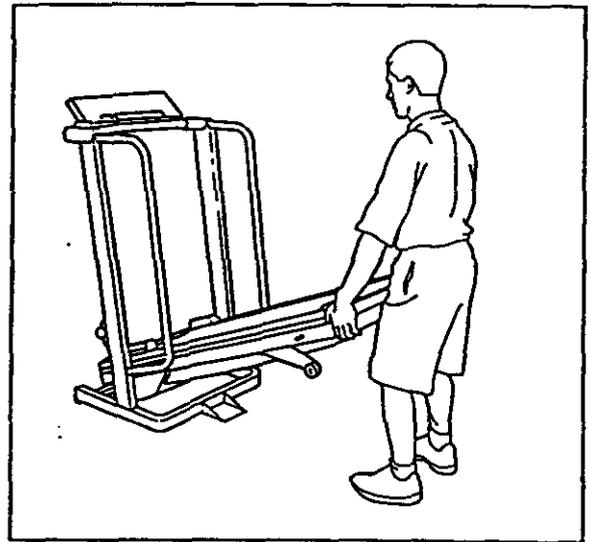
2. Move your right hand to the position shown at the right, and hold the treadmill firmly. Using your left hand, lift the storage latch. Raise the treadmill until the locking pin snaps into the storage latch. Make sure that the locking pin is inside the storage latch, and that the storage latch is fully closed.
