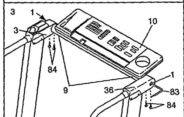
Rotate the Console (10) upward until it stops. Using the 7/32" end of the Allen Wrench (83), tighten the Crossbar Bolts (1) in the ends of the Console Crossbar (9).
