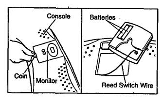
To remove the monitor from the console, gently pry up the monitor with a coin as shown above. Remove the two old batteries from the monitor, and insert two new batteries. Make sure that the negative (-) ends of the batteries are touching the springs, and that the positive (+) ends of the batteries are pushed against the metal contacts.
