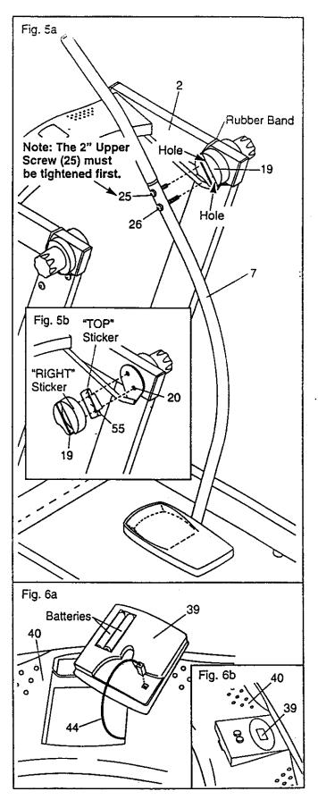
Before you use the AIR WALKER, use the included allen wrench to firmly re-tighten all of the screws used in assembly. Remove the orange and green identification stickers from the AIR WALKER. Note: During the first few minutes that the AIR WALKER is used, a squeaking noise may be heard. This is normal during the break-in period.
