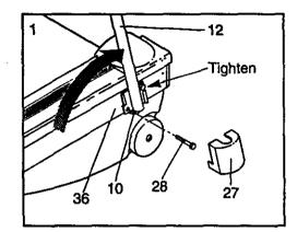
2. Using the 7/32" Allen Wrench (9), loosen the Handrail Bolt that is under the Console (6). Rotate the Console to the position shown. Insert the upper end of the Left Handrail (1) into the left side of the Console. Insert a Handrail Bolt (2) into the bottom of the Console and the Left Handrail (1). Finger tighten the Handrail Bolt.
