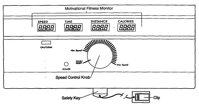
The heart of the treadmill is the innovative console. The console features a safety key-operated power switch, electronic speed control and four independent displays to provide continuous exercise feedback. Please read these instructions carefully before operating the console. Note: If there is a sheet of protective plastic on the face of the console, peel it off before operating the console.
