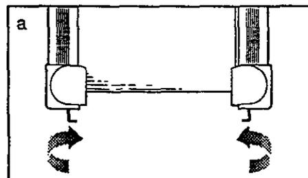
b. If the walking belt has shifted to the right, first remove the key and **UNPLUG THE POWER CORD**. Using the 3/16" allen wrench, turn the left rear roller adjustment bolt counterclockwise, and the right bolt clockwise, 1/4 of a turn each. Be careful not to overtighten the walking belt. Plug in the power cord, insert the key and run the treadmill for a few minutes. Repeat until the walking belt is centered.
