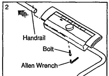
Remove the right handrail cap and the bolt from the lower end of the right handrail. Loosen the other bolt in the handrail (see drawing 3). Lay the right handrail on the treadmill.
