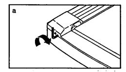
b. If the walking belt has shifted to the right, first remove the key and UNPLUG THE POWER CORD. Using the 3/16" allen wrench, turn the left rear roller adjustment bolt counterclockwise 1/4 of a turn. Plug in the power cord, insert the key and run the treadmill for a few minutes. Repeat until the walking belt is centered.
