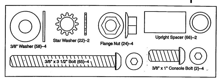
Hold an Upright Spacer (66) inside the lower end of the right Upright (11). (Note: Refer to the inset drawing to identify the right Upright. The Upright Plugs [88] must be on the indicated side.) Insert a 3/8" x 3 1/2" Bolt (65), with a 3/8" Washer (58), into the lower hole in the Upright and through the Upright Spacer. Slide a Star Washer (22) onto the Bolt. Insert a 3/8" x 3 1/2" Bolt (65), with a 3/8" Washer (58), into the other hole near the lower end of the Upright.
