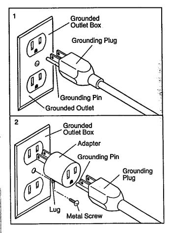
The temporary adapter should be used only until a properly grounded outlet (drawing 1) can be installed by a qualified electrician.
