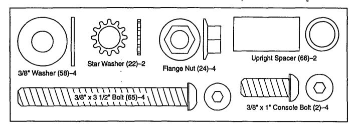
Hold an Upright Spacer (66) inside the lower end of one of the Uprights (11). Insert a 3/8" x 3 1/2" Bolt (65), with a 3/8" Washer (58), into the lower hole in the Upright and through the Upright Spacer. Slide a Star Washer (22) onto the Bolt. Insert a 3/8" x 3 1/2" Bolt (65), with a 3/8" Washer (58), through the other hole near the lower end of the Upright.
