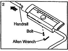
Remove the right handrail cap and the bolt from the lower end of the right handrail. Loosen the other bolt in the handrail (see drawing 3). Lay the right handrail on the treadmill.
