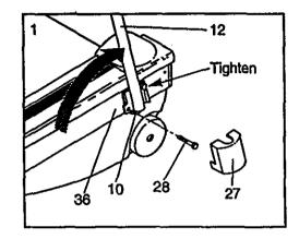
2. Using the 7/32" Allen Wrench (9), loosen the Handrail Bolt that is under the Console (6). Rotate the Console to the position shown. Insert the upper end of the Left Handrail (1) into the left side of the Console. Insert a Handrail Bolt (2) into the bottom of the Console and the Left Handrail (1). Finger tighten the Handrail Bolt.
