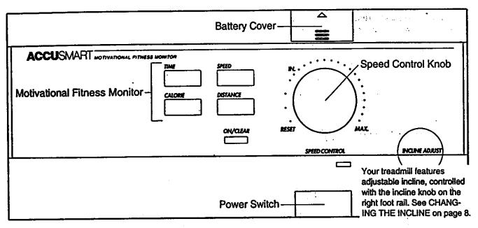
The CROSS WALK features the innovative ACCUS-MART console, designed to help you get the most from your workouts. Please read the instructions below before operating the console. Note: If there is a thin sheet of clear plastic on the face of the console, remove it before operating the console.
