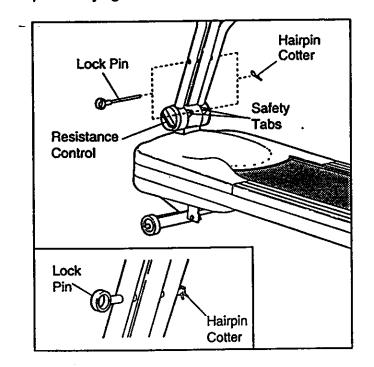
To use the upper body arms in the dual motion position, first make sure the resistance control is firmly tightened. Remove the lock pin from the upper body arms and the upright, and insert it through the safety tabs at the base of the upright. Insert the hairpin cotter into the lock pin.
