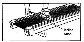
To increase the incline, stand with your left foot towards the back of the left foot rail as shown below. Using your right foot, press down the incline knob on the right foot rail, until the desired incline is reached. To decrease the incline, stand with your left foot towards the front of the left foot rail, and press down the incline knob until the desired incline is reached.
