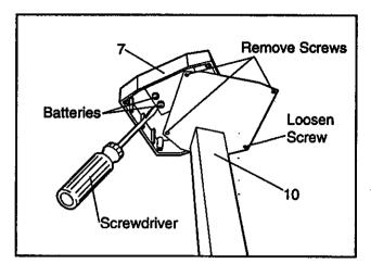
Using a small screwdriver, push the batteries out of the Console (7). Be sure to note which way the batteries were turned. Insert two new batteries. Reattach the Console to the Upright (10).
