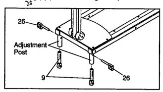
Position the Incline Leg (9) at the desired height, align one of the holes in the Incline Leg with the hole in the adjustment post, and insert the Incline Pin (26) through the adjustment post and the Incline Leg. Adjust the other Incline Leg in the same manner.
