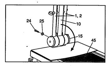
Next, remove the Upright Bolt (24) and Upright Flat Washer (25) from the Upright (10). Lay the Upright and the Upper Body Arms (1, 2) on the Walking Belt (45). Be careful not to pinch the sensor wire in the Upright. Replace the Upright Bolt and Upright Flat Washer for storage.
