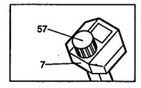
Speed Control is turned clockwise, the resistance on the walking belt will increase and your walking speed will decrease. As the Speed Control is turned counterclockwise, the resistance will decrease and the walking belt will move more freely.
