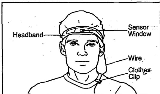
**IMPORTANT:** To avoid static build-up that may damage the console, wear the pulse sensor only while you are on the treadmill.
