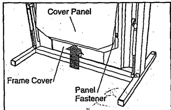
After the cover panel is removed, the panel fasteners can be removed for a cleaner appearance. Using a phillips head screwdriver, remove one of the panel screws and panel fasteners from the frame cover. Tighten the panel screw back into the frame cover. Repeat this process, removing one panel fastener at a time, until all six panel fasteners are removed. Press the removed panel fasteners onto the fasteners on the back of the cover panel. Store the cover panel away from moisture and dust.
