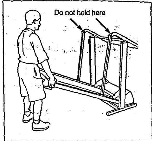
2. Move your right hand to the position shown and hold the treadmill firmly. Raise the treadmill until the storage latch closes over the frame guide. Make sure that the storage latch closes fully over the frame guide.
