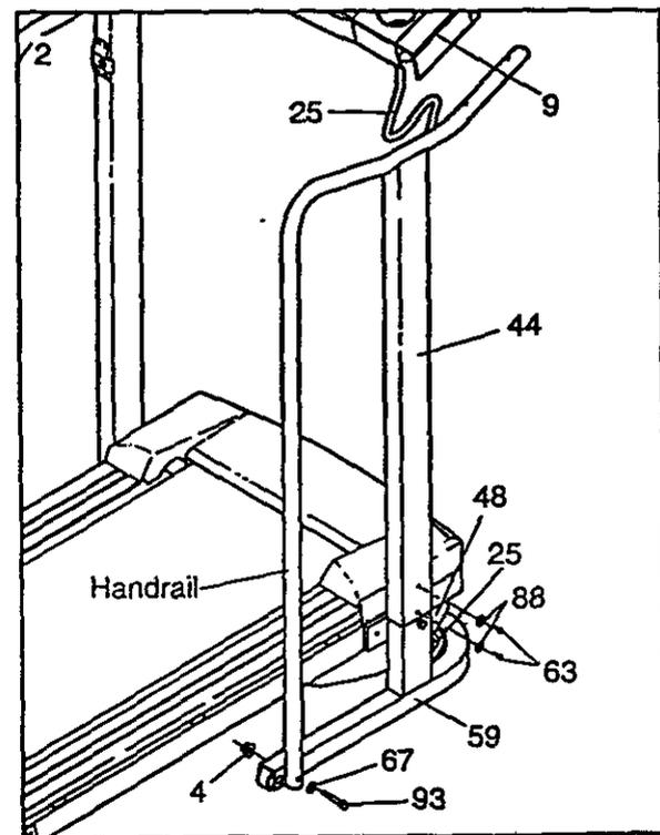
Hand tighten the Handrail Nuts (4) used in steps 1 and 2. Using a wrench, tighten the Handrail Bolts (93) used in steps 1 and 2.
