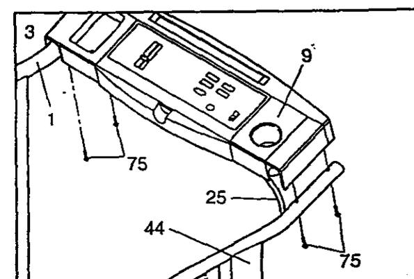
4. With the help of a second person, carefully lower the Left and Right Uprights (1, 44) until the handrails are resting on the floor.
