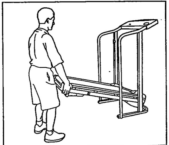
2. Move your right hand to the position shown and hold the treadmill firmly. Raise the treadmill until the storage latch closes over the frame guide. Make sure that the storage latch closes fully over the frame guide.
