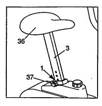
hold the Seat and unscrew the Seat Knob (37). Align one of the holes in the Seat Post (3) with the hole in the Frame (1). Insert the Seat Knob (37) into the Frame and the Seat Post, and tighten the Seat Knob into the Frame. Make sure to insert the Seat Knob through one of the holes in the Seat Post; do not insert the Seat Knob under the Seat Post.
