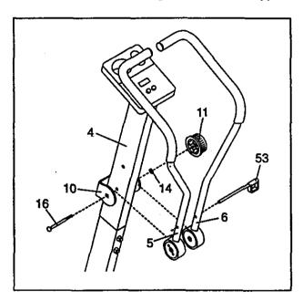
Remove the Lock Pin (53). Turn the Resistance Dial (11) counterclockwise and remove it. Remove the M10 Star Washer (14). Using pliers, grip the head of the 3/8" x 6" Carriage Bolt (16) and remove it. Apply a thin film of grease to both sides of the Handlebar Housings (72). Reattach all parts, making sure that they are in the positions shown.
