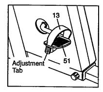
Pedal Strap onto the adjustment tab.
