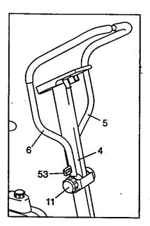
Post. Note: If it is difficult to insert the Lock Pin, twist the Handlebars slightly in order to align the holes. Next, tighten the Resistance Dial (11) (see the drawing above).
