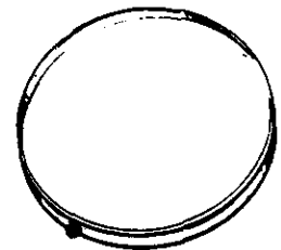
DRAIN PANS AVAILABLE IN 20" DIAMETER FOR WATER HEATERS HAVING A DIAMETER 18" OR LESS AND AVAILABLE IN 28" DIAMETER FOR WATER HEATERS HAVING A DIAMETER 26" OR LESS
