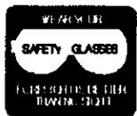
The operation of any tiller can result in foreign objects thrown into the eyes, which can result in severe eye damage. Always wear safety glasses or eye shields before starting your tiller and while tilling. We recommend a wide vision safety mask over spectacles or standard safety glasses.
