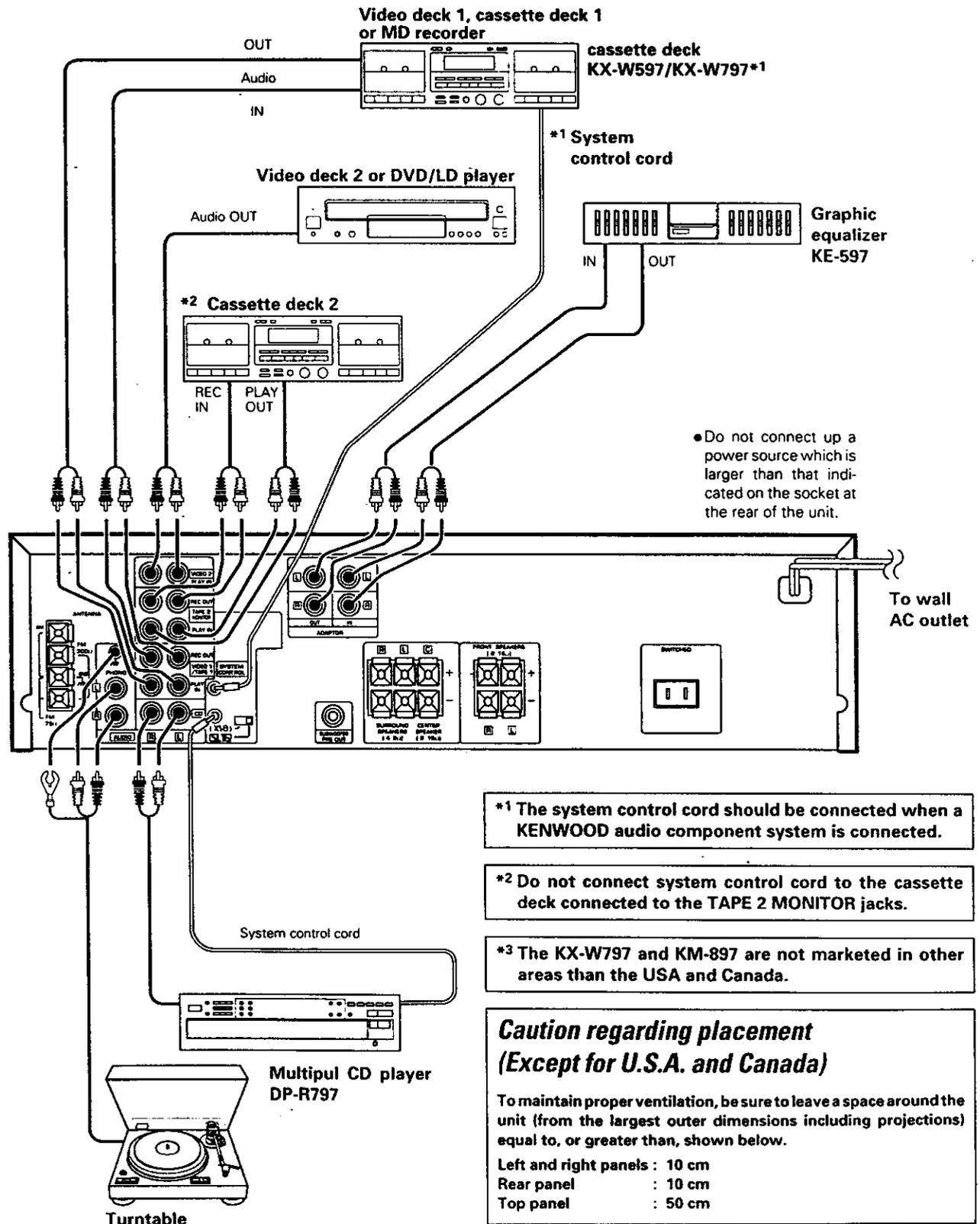
● Do not connect up a power source which is larger than that indicated on the socket at the rear of the unit.
