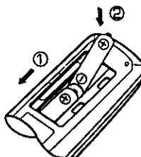
● Insert two AA-size (R6 / SUM-3) batteries as indicated by the polarity marking.
