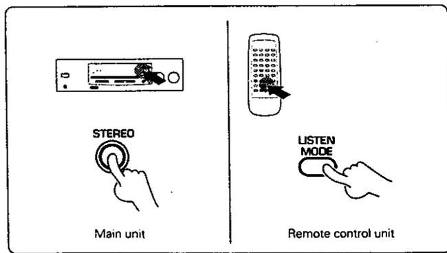
On the remote control unit, the following modes are switched every time the LISTEN MODE key is pressed.
