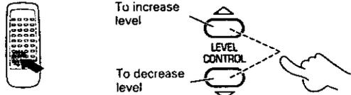
The level can be adjusted between -8 and +8 with an increment or decrement of 2 per press.
