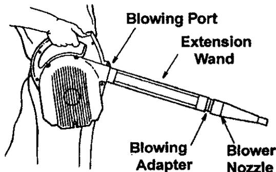
3. Turn the blower “ON” by toggling the switch in the handle of the blower to the “ON” position.
