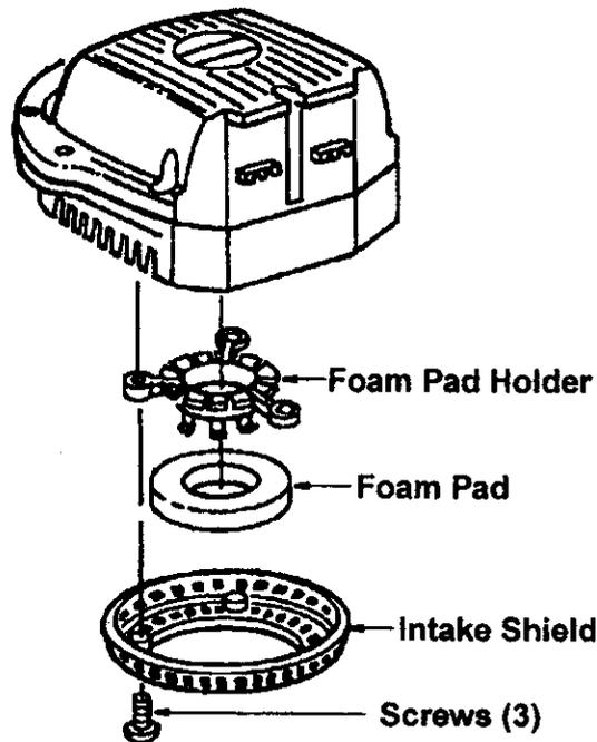
6. Replace foam pad holder on blower with the tabs away from the blower. Reinstall foam pad under the tabs of the holder.
