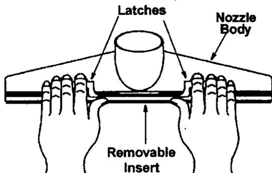
2. Using both hands, position each thumb on the removable insert, (below the latches) and two fingers of each hand on each latch, lift and disengage the two latches from the tabs on the nozzle body.
