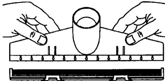
3. Press down with each thumb below the latching tabs until you see and hear the removable insert snap into the nozzle body. Snap the latches over the locking tabs into their original position.
