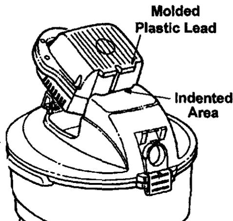
3. Rotate the detachable blower down until the travel of the unit stops.
