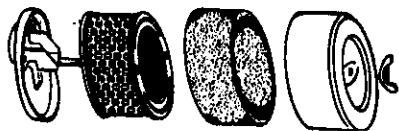
Base Plate Inner Paper Filter Outer Foam Filter Cover and Wing Nut
