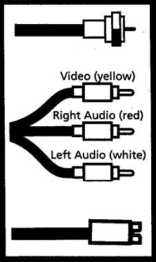
Coaxial Cable is the standard cable that comes in from your antenna or cable box. Coaxial cables use "F" connectors.
