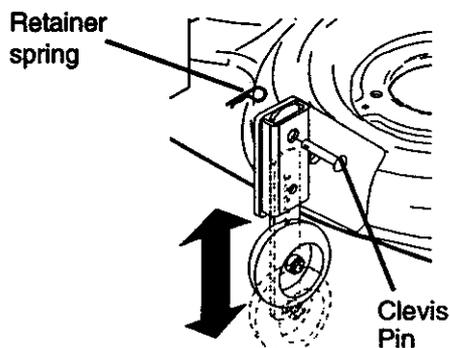
**IMPORTANT:** Be sure to readjust gauge wheels if you change the cutting height of the mower deck.
