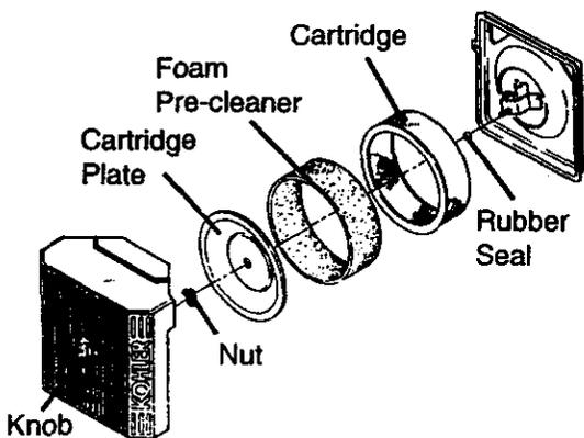
**NOTE:** Do not wash the paper cartridge or use pressurized air, as this will damage the cartridge.
