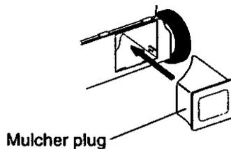
**▲CAUTION:** Do not run your lawn mower without mulcher plug in place or approved clipping deflector or grass catcher in place. Never attempt to operate the lawn mower with the rear door removed or propped open.
