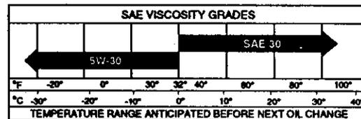
**NOTE:** Although multi-viscosity oils (5W30, 10W30 etc.) improve starting in cold weather, these multi-viscosity oils will result in increased oil consumption when used above 32°F. Check your engine oil level more frequently to avoid possible engine damage from running low on oil.
