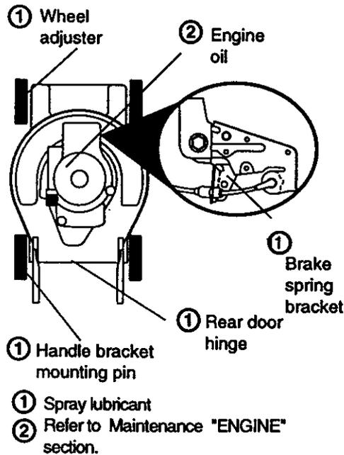
**IMPORTANT:** Do not oil or grease plastic wheel bearings. Viscous lubricants will attract dust and dirt that will shorten the life of the self lubricating bearings. If you feel they must be lubricated, use only a dry, powdered graphite type lubricant sparingly.
