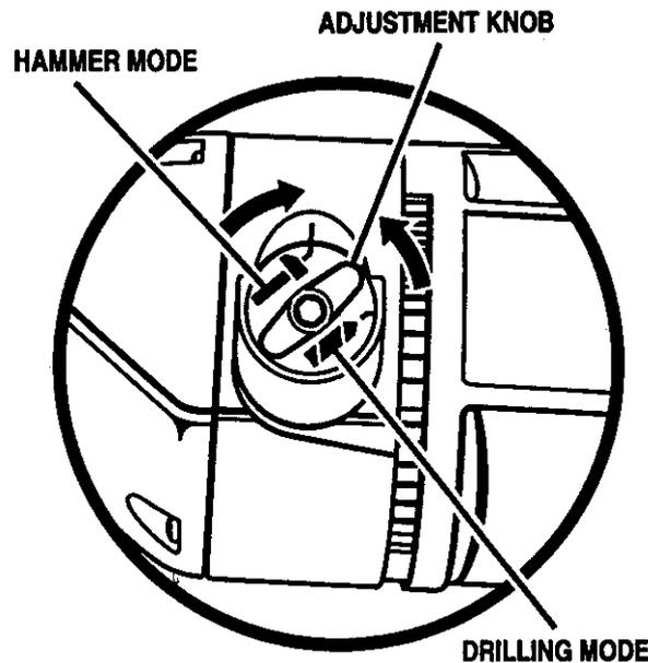
We recommend that you use carbide-tipped bits and select hammer mode when drilling in hard materials such as brick, tile, concrete, etc.
