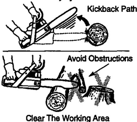
**WARNING:** Rotational Kickback can occur when the moving chain contacts an object at the upper portion of the tip of the guide bar. Contact at the upper portion of the tip of the guide bar can cause the chain to dig into the object, which stops the chain for an instant. The result is a lightning fast, reverse reaction which kicks the guide bar up and back toward the operator.
