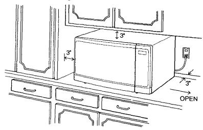
1. Select a level surface that provides enough open space for the intake and/or outlet vents.
