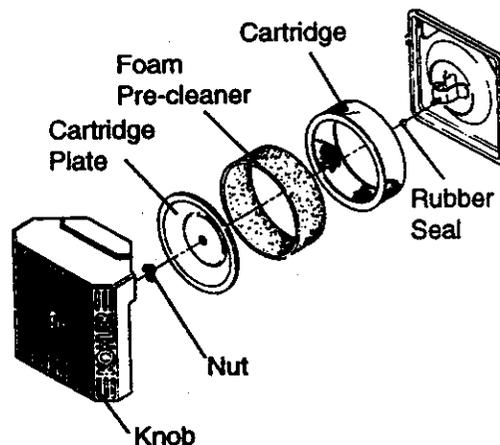
**NOTE:** Do not wash the paper cartridge or use pressurized air, as this will damage the cartridge.
