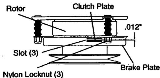
**NOTE:** After installing a new electric clutch, run tractor at full throttle and engage and disengage electric clutch 10 cycles to wear in clutch plate.
