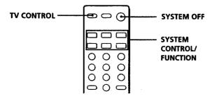
Press one of the SYSTEM CONTROL/FUNCTION buttons to select the component you want to use. The SYSTEM CONTROL/FUNCTION buttons on the remote are factory-set as follows:
