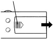
Place two "AA" size batteries, matching the + and – signs on each battery to the + and – signs of the battery compartment.
