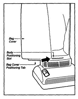
Be sure bottom of dust bag is completely within bag cavity prior to replacing the bag cover.
