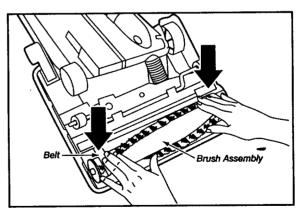
Press firmly, checking to see that each end is completely inserted.
