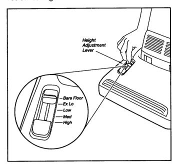
In this position, the headlight is off and the brush assembly does not revolve. This setting is recommended for cleaning hardwood and tile floors.
