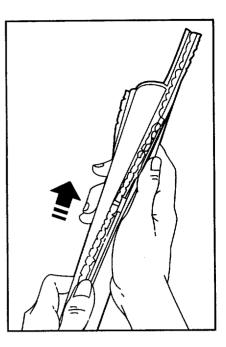
in warm water for a few minutes before sliding them into the slots. Do not use oil. Dry thoroughly before reinstalling.
