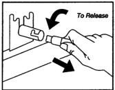
Pull the light bulb to remove.
