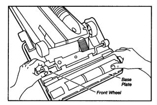
On the right side, lift the latch hook slightly to place the base plate into position. The base plate will not close unless the base plate is under the latch hook.
