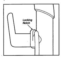
Lock the cord into place by forcing it into the locking notch on the body of the upper cord hook as shown. This helps keep the power cord out from under the vacuum cleaner brush assembly.
