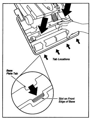
As the base plate is lowered, the left side will brush against the front wheel.
