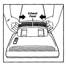
Grasp the air exhaust panel with a hand on each side, press inward and pull the panel forward. Lift the foam filter to remove. Wash the foam filter, rinse and dry.
