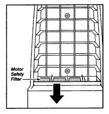
If the foam Motor Safety Filter located at the base of the bag cavity is dirty, remove it by pulling forward.
