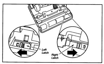
To unlock the base plate, slide the left latch to the left and the right latch to the right.
