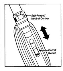
To start the vacuum cleaner, slide the On/Off Switch to the ON position. Use the OFF position when leaving or storing the cleaner.
