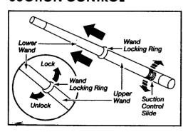
Attach the extension wand onto the open end of the hose.
