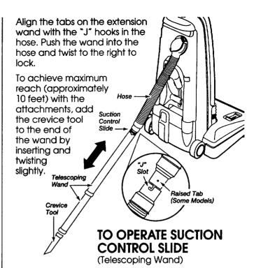
When using attachments for cleaning draperies, small rugs with low pile and other delicate items, twist the Suction Control Lever to the open position. This lever is located on the Telescoping Wand, close to the hose.
