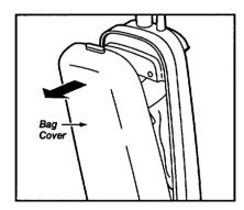
Pull the bag cover forward. Remove and lay aside.
