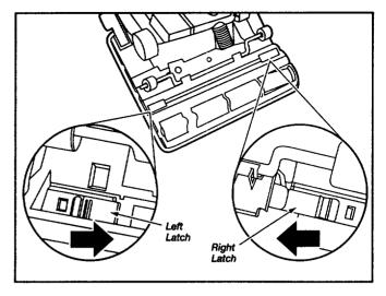
Slide latches toward the center of the unit to secure.
