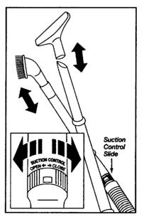
When using the dusting brush or the upholstery tool, they may be attached directly to the wand or placed on the end of the crevice tool.
