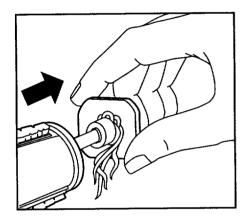
Carefully remove the brush end caps and metal washers to check for string and hair build-up.
