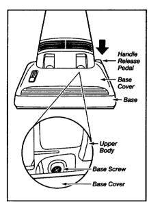
Press the handle release pedal to let the upper portion of the cleaner lay back against the floor.
