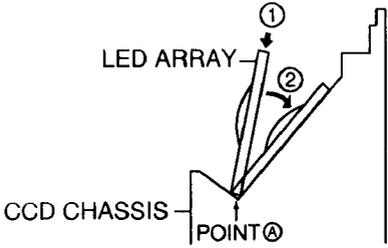
**Note:** Place the LED Array in the center of point A as shown above.
