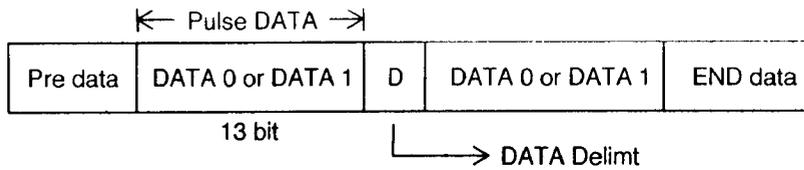
When executing Pulse Dial, the Pulse Dial DATA is transmitted from the Portable Handset to the Base Unit in above format. The combination of DATA 0 and DATA 1 are changed by each Dial No. And the DATA Delimt is between each Frame as a stop. The number of Frame is 2.
