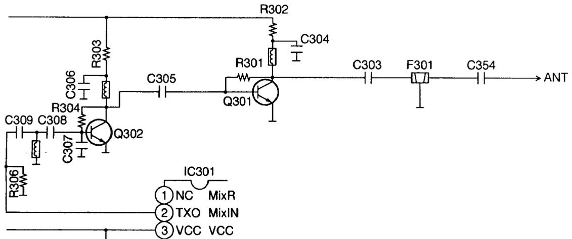
(6) Second Mixer, Detector, Carrier Sense Circuit ( ): Portable Handset
