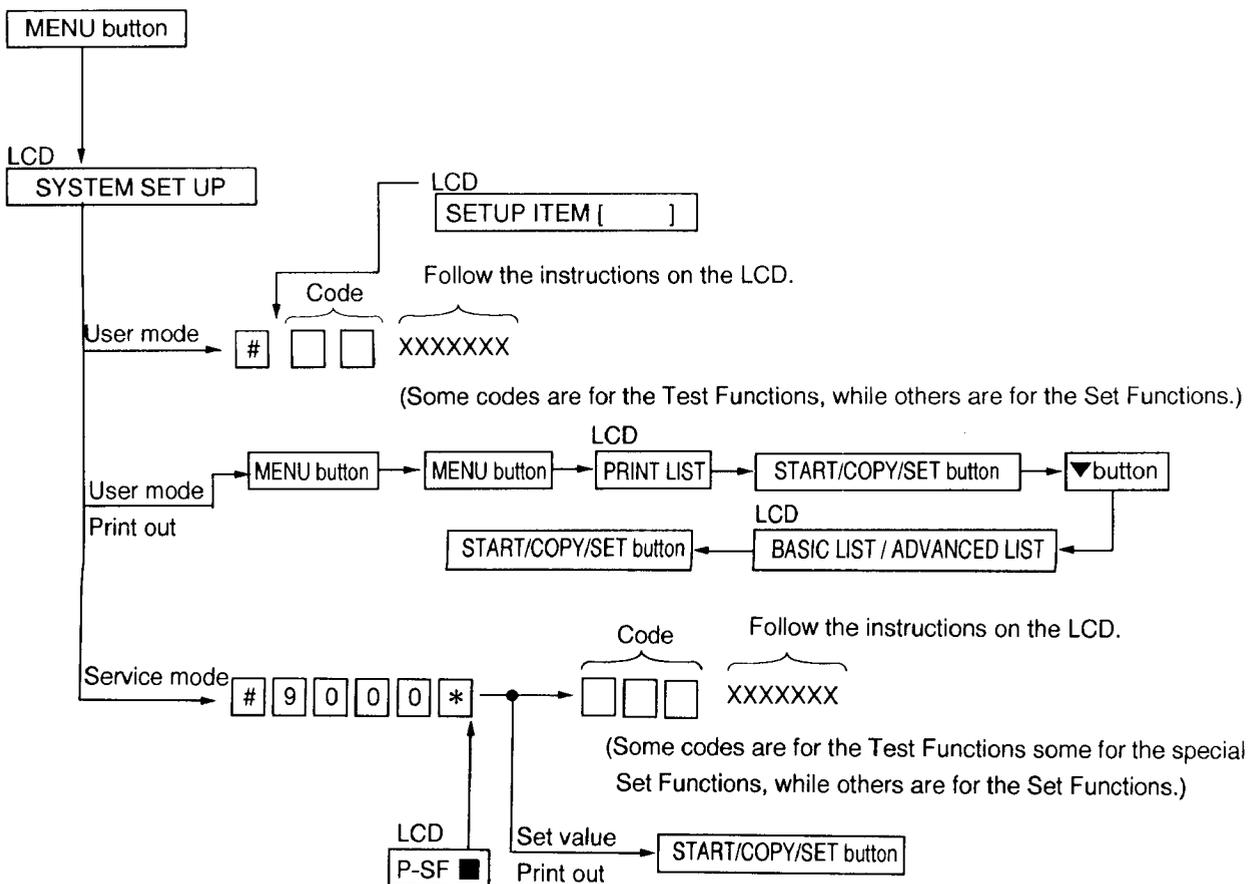
4-3. USER MODE (The list below is an example of the SYSTEM SETUP LIST the unit prints out.)
