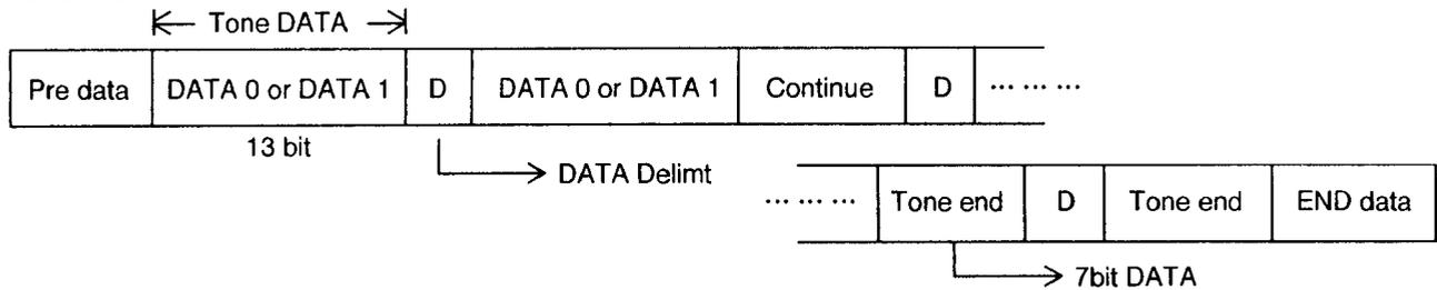
When executing Tone Dial, Tone Dial DATA is transmitted from the Portable Handset to the Base Unit in above format. The DATA is changed by Dial No. as same as Pulse Dial. When Tone Dialing, DATA (Continue DATA) that the key is pressed continuously is sent to the Base Unit during the key is pressed. When depressing the key, the TONE Dial exterminating DATA (Tone end DATA) is send, and the END data is sent finally.
