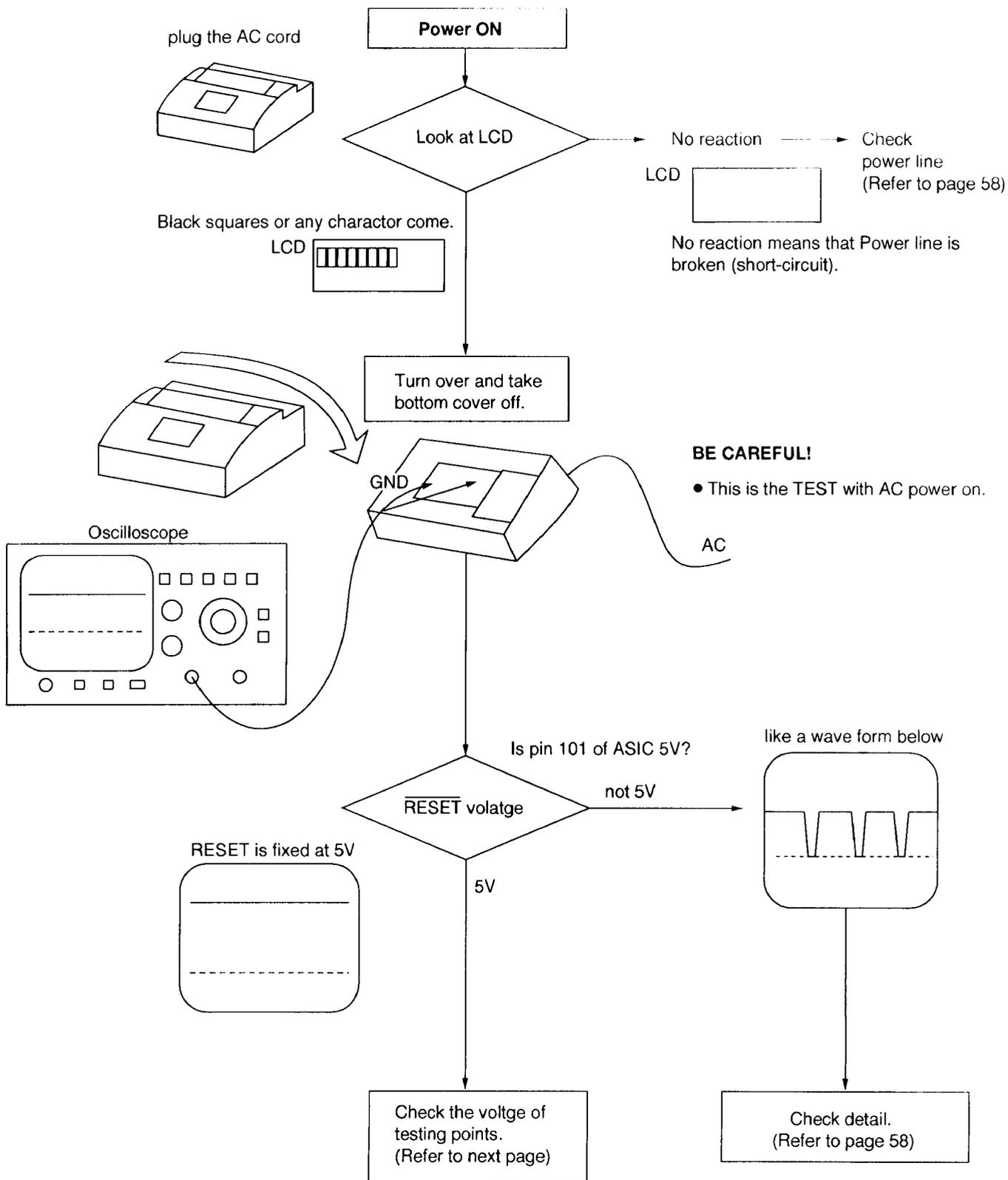
Please check the status (voltage) of pin 56, pin 58 and pin 60 of IC1.
