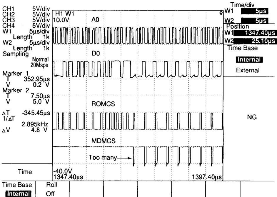
Below graph show you the wave form that is observed when SRAM doesn't work. (BUS line at SRAM is intentionally opened.) Please compare OK (under) to NG (upper). SRAMCS (pin 20 of IC3) signal is coming like clock. In the case of this wave form SRAM access doesn't work. If soldering, conductance is no problem, we need to replace SRAM (IC3).
