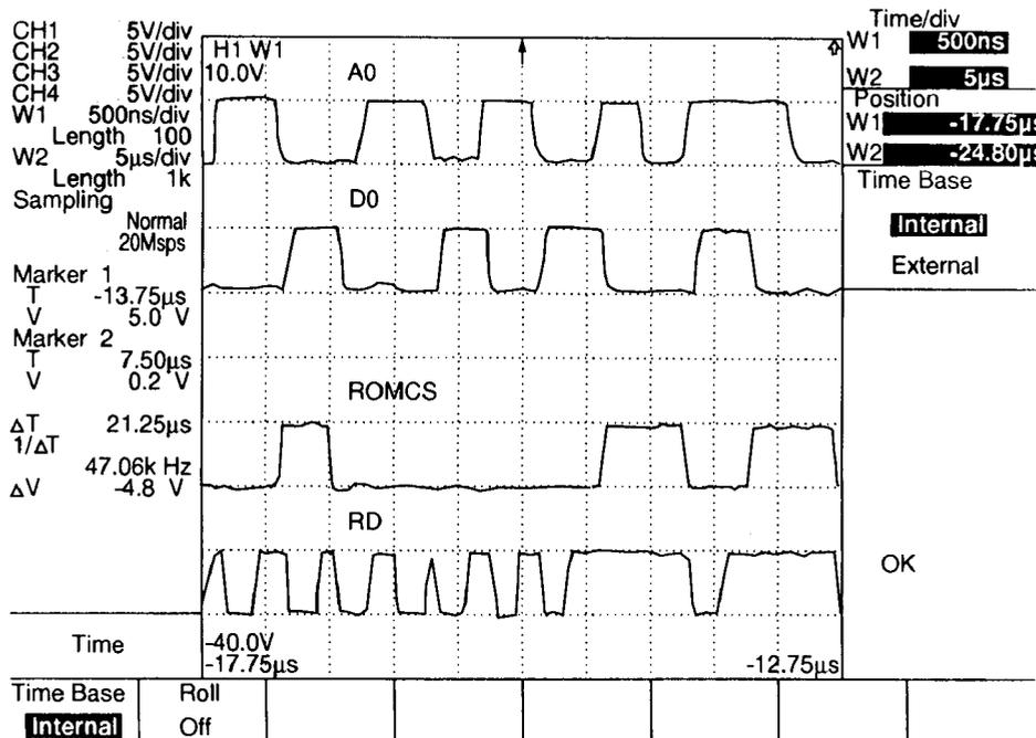
The graphs below show you the wave form that is observed when unit (board) doesn't work. (A3 is intentionally opened at pin 135 of ASIC in this board.)
