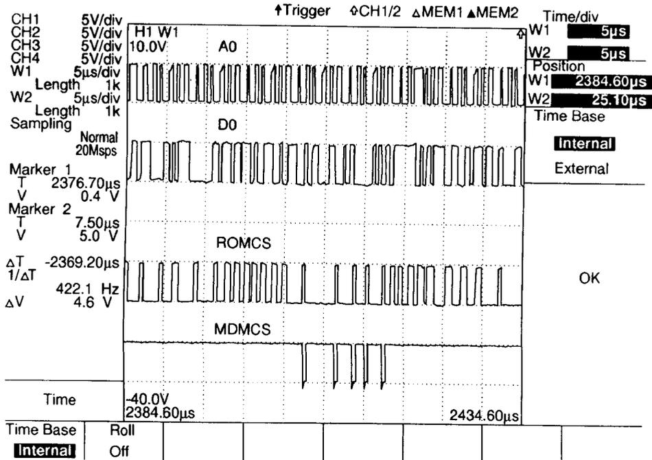
The graphs below show you the wave form that is observed when MODEM doesn't work. (Oscillation is not intentionally supplied to MDM.)
