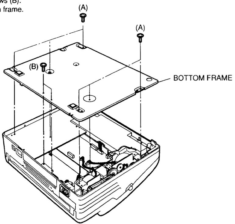
Ref. No. 5 **HOW TO REMOVE THE ANALOG, DIGITAL BOARDS, SPEAKER AND MIC**
