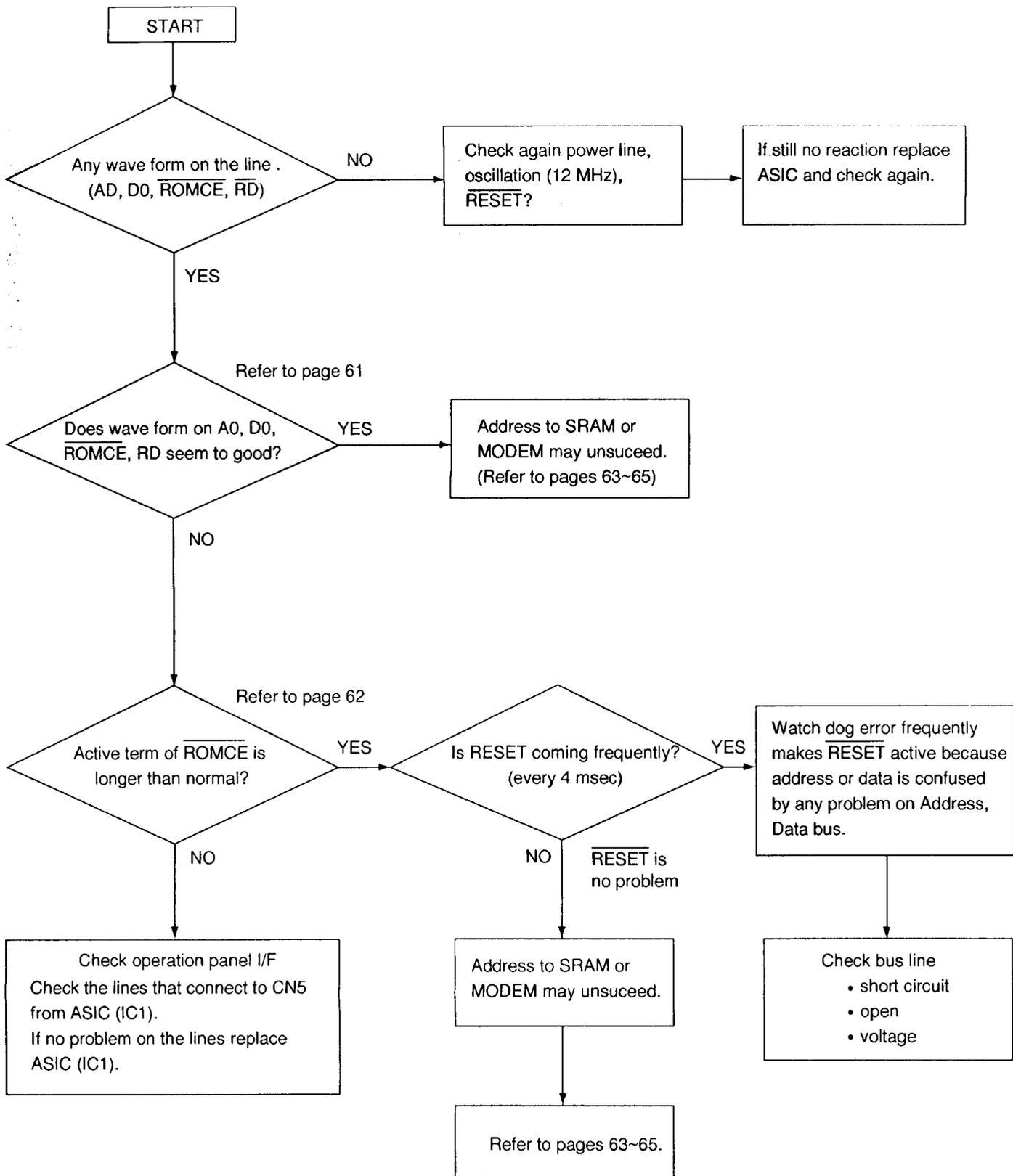
Let's observe the wave form to fix the defective IC.
