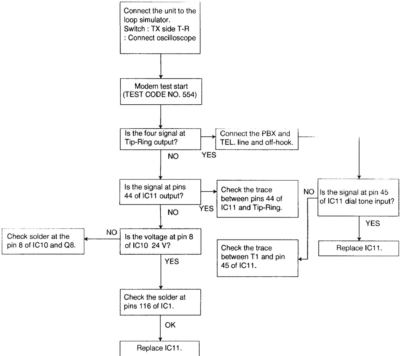
④ Unit can copy, but can not transmit/receive long distance or international communication
