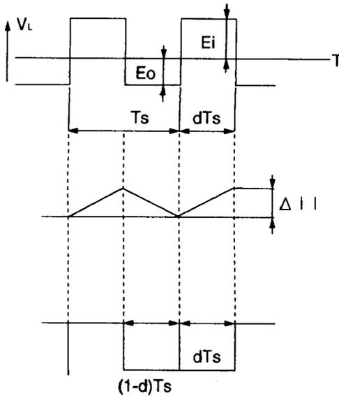
In the actual circuit, the fixed output voltage can be obtained by changing the winding ration of transformer T101. In this converter circuit, the duty ratio of ON period and OFF period of the transistor produces output. In this power supply, the bias winding is also built-in in the transformer and the output value is one. 24V output voltage is stabilized and changes the duty ratio.
