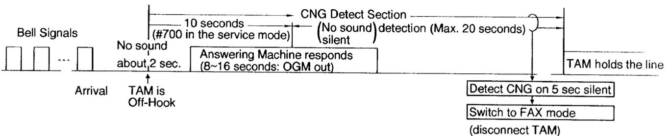
**Attention 1:** No sound detection lasts 20 seconds after the telephone call coming in to the answering machine. If there is no sound situation for more than 5 seconds (#701 in the service mode) it is switched to the facsimile.
