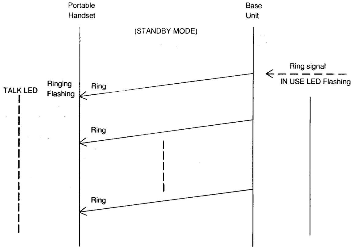
After detecting the Ring signal from circuit, Base Unit sends a ring signal DATA (Ring), then the Portable Handset starts ringing.
