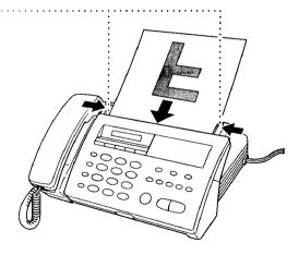
■ The automatic document feeder (ADF) can hold up to 10 pages, feeding each one individually through the fax machine. Use standard (20 lb.) paper when using the ADF; if you're using heavier paper, feed each sheet individually to prevent paper jams.
