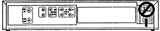
Do not plug TV into switched outlet on a VCR or cable-TV decoder
