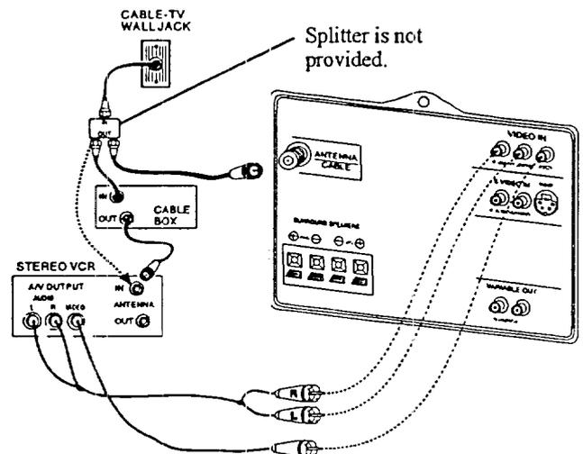
Required Cable-TV Connection For Use With PIP
