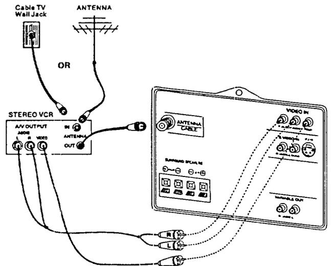
Required Antenna Connection For Use With PIP
