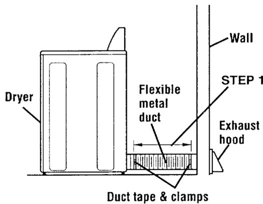
Cut 2 inches longer than measurement to fit over dryer and hood connections.
