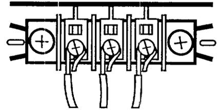
**STEP 5.** Connect the other two wires to outer terminal block screws using the same method(s) described in STEP 4a. Tighten all terminal block screws firmly.
