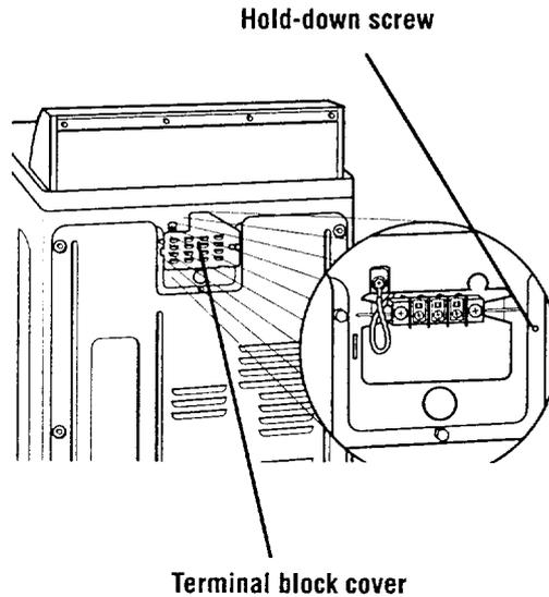
**STEP 3.** Attach  $\frac{3}{4}$ " U.L.-listed strain relief (U.L. marking on strain relief) to the hole below terminal block opening. Put the direct wire cable through the strain relief.
