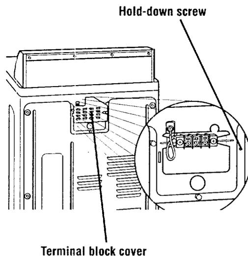
**STEP 3.** Attach  $\frac{3}{4}$ " U.L.-listed strain relief (U.L. marking on strain relief) to the hole below terminal block opening. Put the power supply cord through the strain relief.
