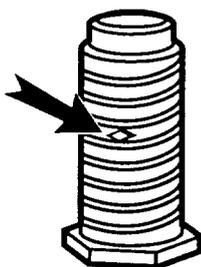
**STEP 4.** Start to screw the legs into the holes by hand. Use an adjustable wrench or other type wrench to finish turning the legs until you reach the diamond marking. Later adjustment may be needed.
