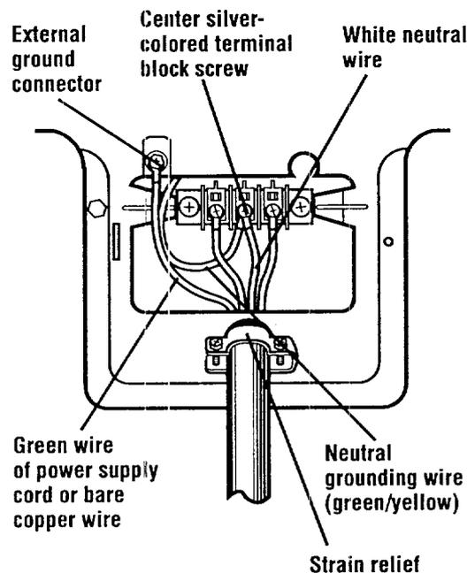
**4-Wire Connection with Frame-Grounding Conductor**
