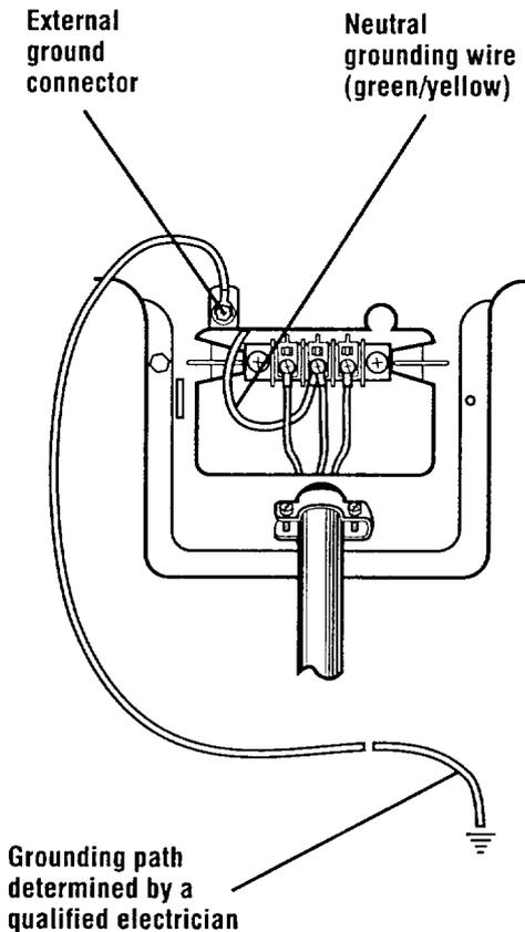
**Alternate 3-Wire Connection with External-Grounding Conductor**
