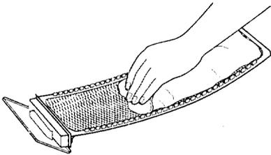
**STEP 3.** Push the lint screen firmly back into place.
