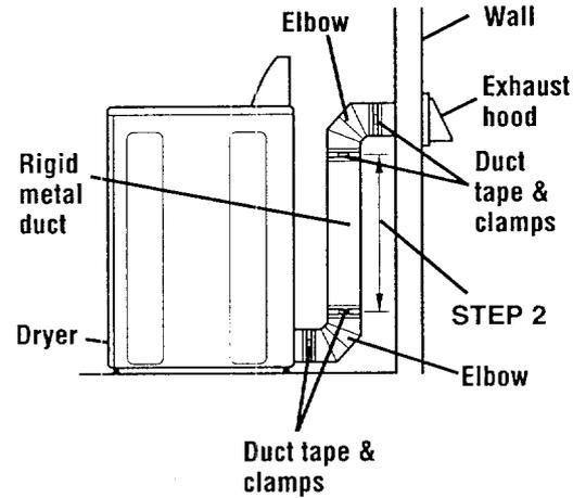
The duct usually comes in 2-foot lengths. Cut 2 inches longer than measurement for connection.
