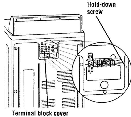
**STEP 3.** Attach 3/4" U.L.-listed strain relief (U.L. marking on strain relief) to the hole below terminal block opening. Put the direct wire cable through the strain relief.
