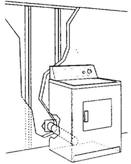
Avoid pushing the dryer tightly against a wall. This can crush or kink the duct. Use the straightest path you can, where possible, to avoid 90° turns.
