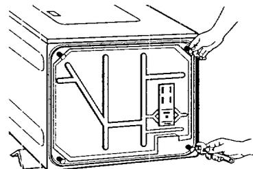
**STEP 5.** Now stand the dryer up. Slide dryer onto cardboard and move dryer close to its final location. Leave enough room to connect the exhaust duct.
