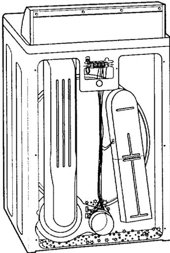
**STEP 3.** Remove lint from the dryer base with a soft brush or vacuum cleaner. Avoid damaging wires or electric thermostats.
