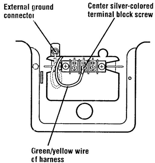
**STEP 5.** Connect neutral grounding wire and the neutral wire (white or center) of direct wire cable under the center screw of terminal block.
