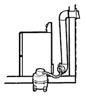
Inspect and clean the dryer exhaust ducting at least once a year to prevent clogging. A partially clogged exhaust can lengthen the drying time.
