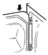
7 Remove the remaining screws from the side of the opening from which the door was removed. With these screws secure each hinge at the bottom.
