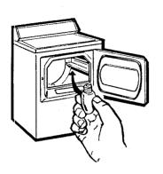
Before replacing the light bulb, be sure to unplug the dryer power cord or disconnect the dryer at the household distribution panel by removing the fuse or switching off at the circuit breaker. Reach above dryer opening from inside the drum. Remove the bulb and replace with the same size bulb.
