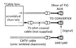
For this set up, you can switch between scrambled channels (through your cable box), and normal (CATV) channels by pressing ANT on your remote cor.trol.
