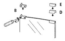
Push the top glass door hinge into the top right bushing and gently slide the glass door into the bottom hinge. Adjust the glass door until level, and tighten the hinge screws.
