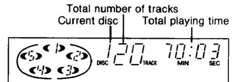
The total playing time displayed includes the silent sections between tracks. For this reason, it may be a few seconds longer than the playing time indicated on the disc.
