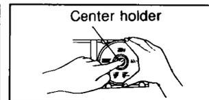
To return the disc to the case, insert the disc with the label facing up and press downward at the center.
